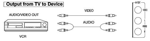
The side terminals may be easier to use with a camcorder. The connections are identical.
